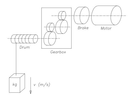
The balance becomes at descent speeds between 10 to 25% higher to the nominal, depending on the load, efficiency of the transmission and temperature of the system.
