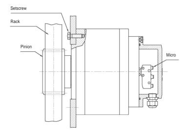
The unit **must be firmly attached to the platform structure** so that the sprocket is perfectly centered and in engagement with the rack. After mounting the unit, connect the cables to the micro connector. Typically, this is in closed position.
