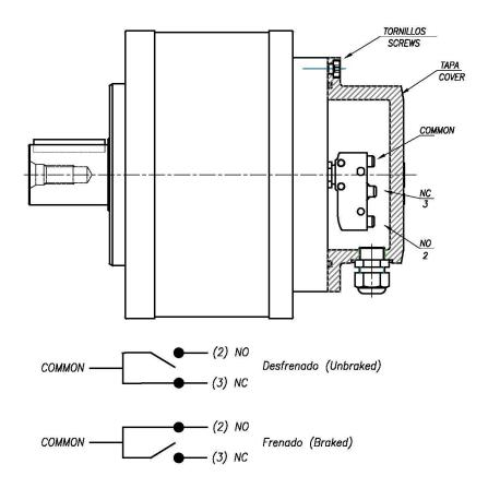
The micro changes state when the brake is locked. The micro recovers its initial position when the brake is released.
