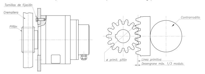
The pinion should cover the entire length of the rack and its disengagement may not be more than 1/3 module at any point.
