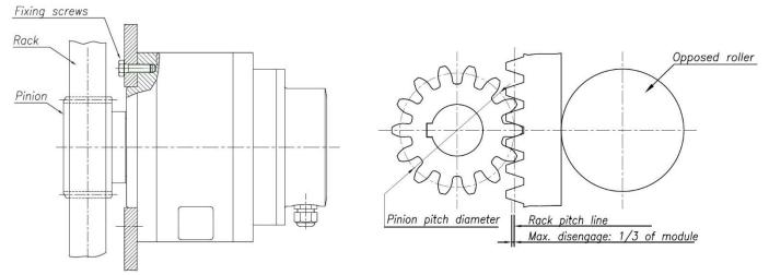
The pinion should cover the entire length of the rack and its disengagement may not be more than 1/3 module at any point.
