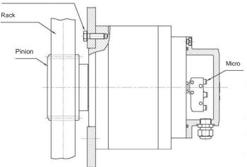
The unit **must be firmly attached to the platform structure** so that the sprocket is perfectly centered and in engagement with the rack. After mounting the unit, connect the cables to the micro connector. Typically, this is in closed position.
